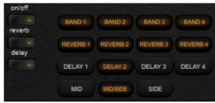
**Band buttons:** These buttons are used to turn on and off the different frequency-ranges. When turned off, it turns off the whole stream of signs from the ranges – meaning that both effects and the original sign will be turned off. In this state the frequency-ranges' interface can't be seen, therefore it's easy to tell which range is on or off.
