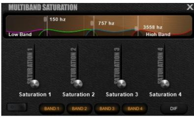
Saturation is a whole new function where the audio sign can be edited in 4 frequency ranges. Using the feature the volume of the overtone sounds can be strengthened, and a more analog tune can be achieved.
